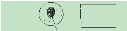
h) Note fatigue lines originate from the internal point, not outer diameter. Very rare failure type due to steel defect. 100% warranty accepted.
