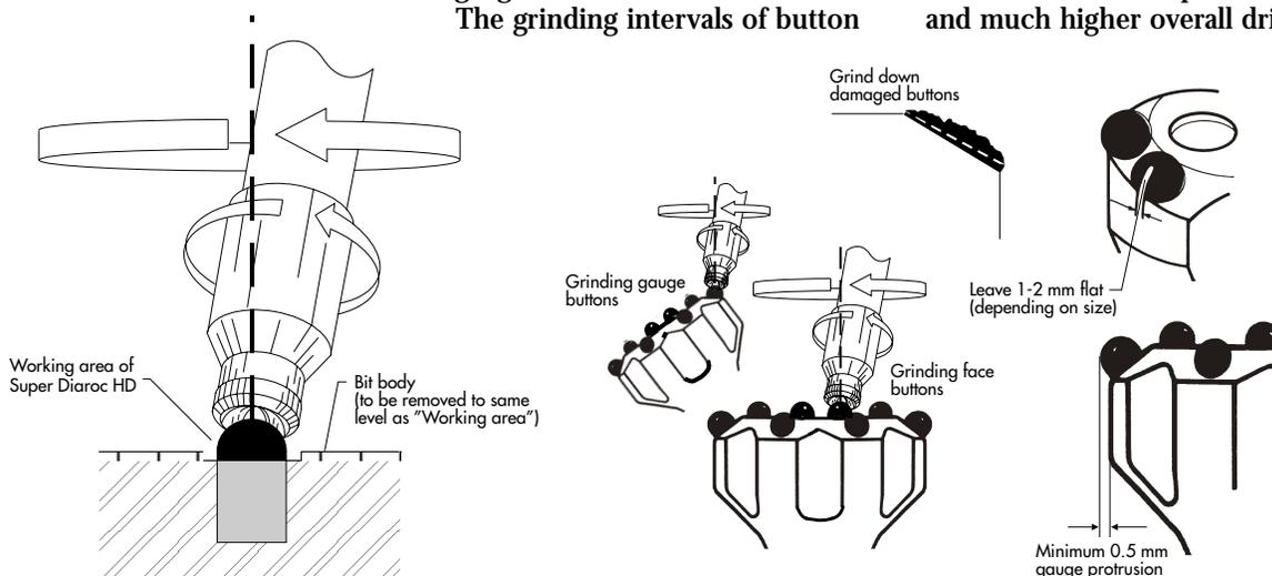
To grind a button correctly, oscillate the grinder in an orbital motion around the axis of the button insert.
